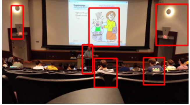
Figure 3. Human Detector Output. By using a low detector threshold we have fewer missed detections of the person-of-interest, but we also have more false positives.
